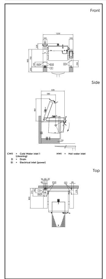
Electric 400 V/3N ph/50/60 Hz Supply voltage: Total Watts: 15.5 kW Installation: FS on concrete base;FS on feet;On base;Standing Type of installation: against wall
